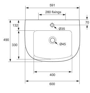
All measurements shown are in millimetres.
